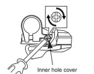
Connect the cable to the rear derailleur and, after taking up the initial slack in the cable, re-secure to the rear derailleur as shown in the illustration.
