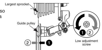
**4. How to use the B-tension adjustment screw**
