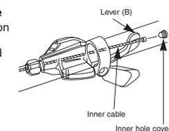
Install the inner hole cover by turning it as shown in the illustration until it stops. Do not turn it any further than this, otherwise it may damage the screw thread.
