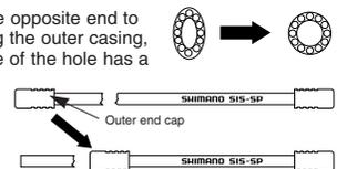
Attach the same outer end cap to the cut end of the outer casing.
