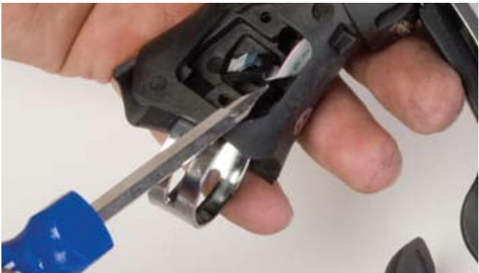
5. To remove the main assembly, move flight deck contacts towards the front passway.
