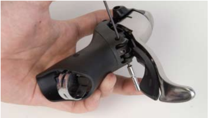
3. Then push to remove the axle.
