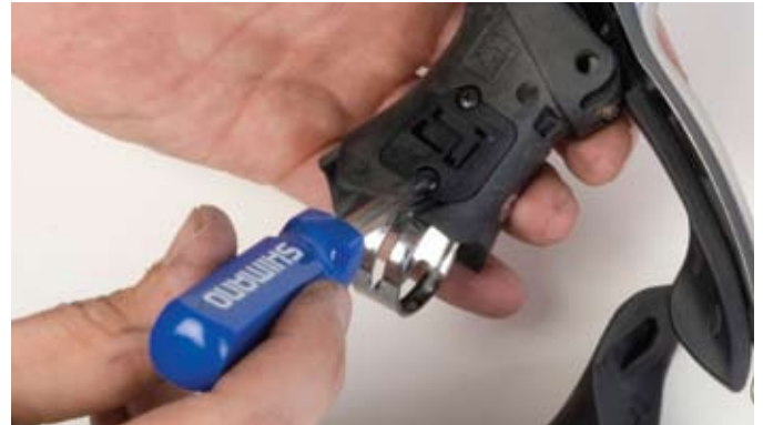
4. Remove flight deck sensor bracket or place holder if sensor is not installed.
