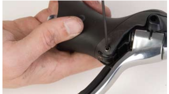
2. Insert Allen key into either end of the axle.
